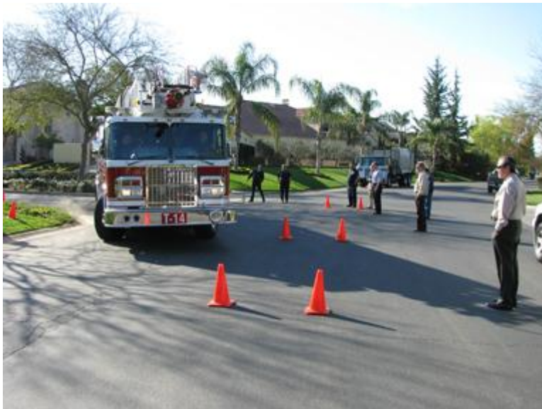
▣ Figure 1 Cones Placed to Simulate Narrower Road Pavements – Fire Truck Navigates Without a Problem
